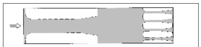
Top view: Exhaust silencer module consisting of (from left to right) very low frequency module, plenum and low/mid frequency module.
