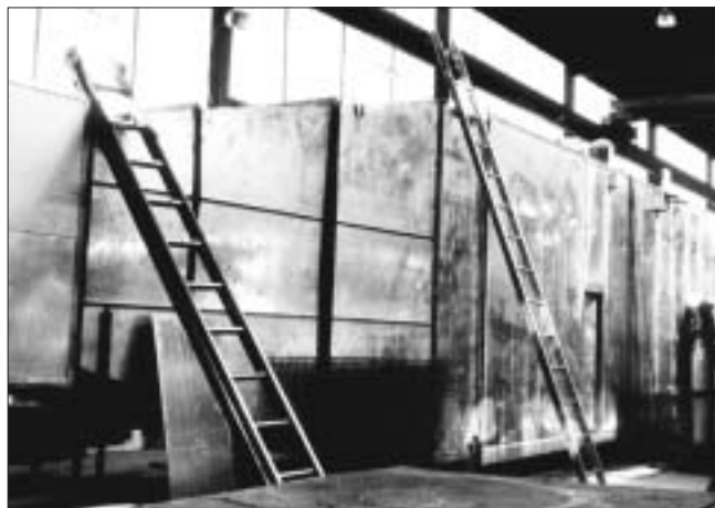
Fan/silencer package and test duct.
