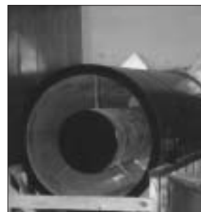
Vibro-Acoustics' conducted full-scale laboratory tests to ensure that the aero-acoustic performance of the large jet fan silencers was achieved.
